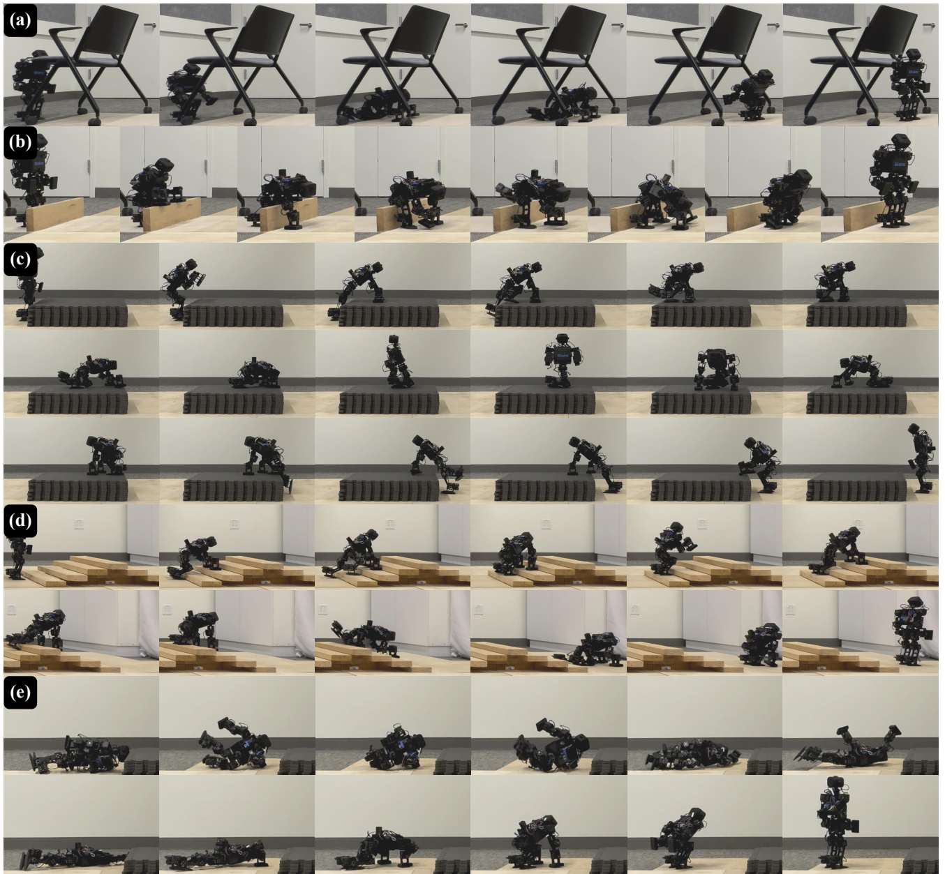
Fig. 4: Terrain Policies. We demonstrate our policies on traversing extremely challenging terrains—including (a) low-clearance spaces under chairs, (b) knee-high walls, (c) knee-high platforms, and (d) steep ascending and descending stairs—and additionally show (e) fall recovery from supine and prone positions in case of failure.
